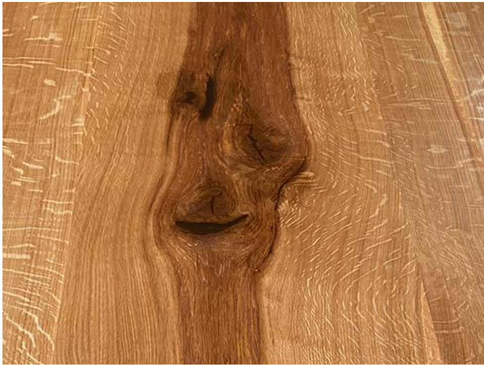
Above: Hardened resin is sanded, stained, and varnished with the rest of the top.
