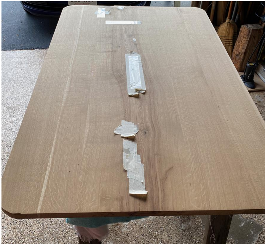
Above: The table that went to daughter Ann had voids that I filled with System 3 resin. Tape on the underside holds resin when clear-through voids needed to be filled.
